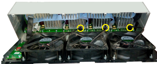
Figure 3: Disconnect the fan wires
